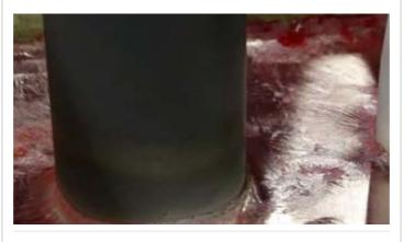
A novel 20 kHz ultrasound generator creating uniformly distributed 3D acoustic energy for degassing, mixing, alloying and homogenization of (molten) aluminium.
