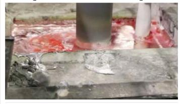
Ultrasonic uniform vibration of the melt caused by a special grade Sialon non-wetting sonotrode
